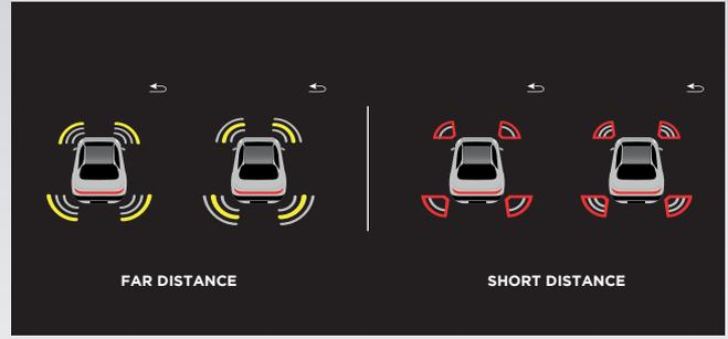
Six ultrasonic sensors are located in the front and rear side to identify vehicles and all static objects nearby that could cause a potential collision.
